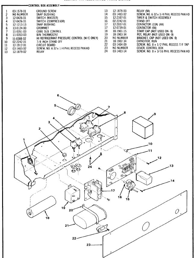
Figure 8-5. CM850 Control Box Assembly.
