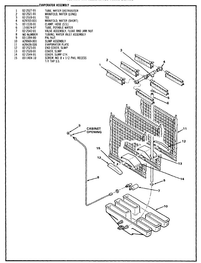
Figure 8-4. CM850 Evaporator Assembly.
